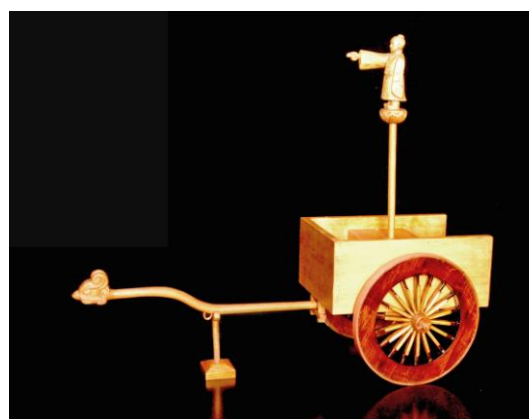
Fig. 1 Mechanical South-pointing Chariot (created by the author)
